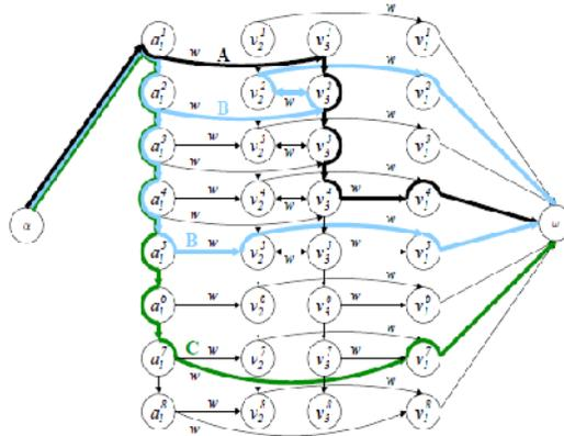
Figure1. A sample DNTG, with one Access point A and three vehicles v1, v2 & v3, the vehicle (v1) is a downloader while the others (v2, v3) can act as relays. In the above graph, we show up paths that are agent of the carry and-forward (A), connected forwarding (B), and direct transfer (C) paradigms.
