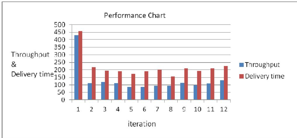
Chart 4 Throughput and delivery time for manufacturing product a in n-supplier model
