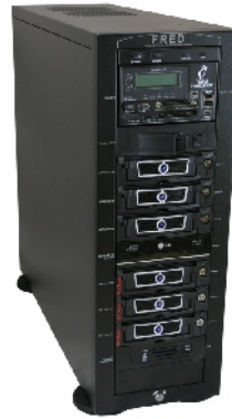
Figure 1 Forensic Recovery of Evidence Device [ HYPERLINK \l "Dig12" 16 ] (FRED)
