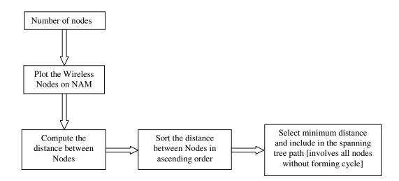
Figure 4. Spanning Tree Construction
