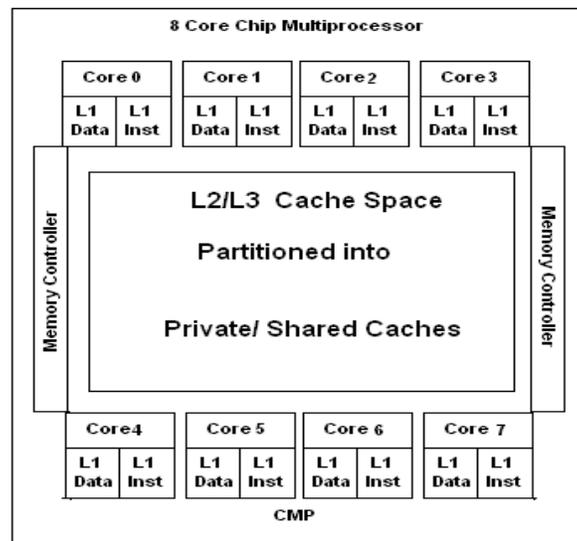
Figure2. Single Chip Multiprocessor (CMP)
