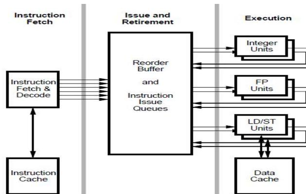
Figure1. Dynamic Super Scalar Microprocessor
