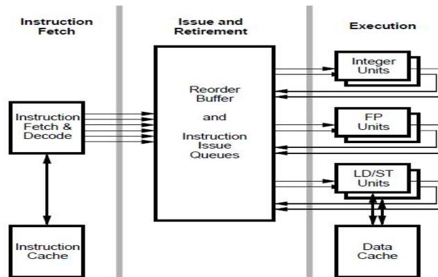
Figure1. Dynamic Super Scalar Microprocessor
