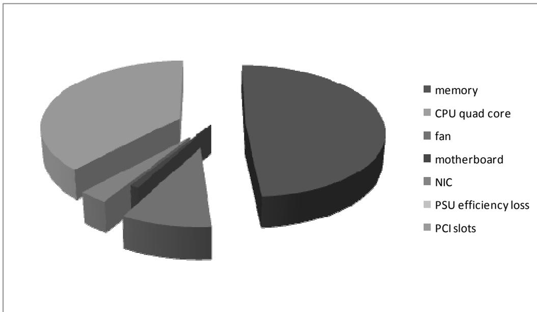
Figure 2.power consumption of the server [26].
