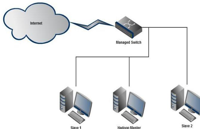
Figure 2: Experimental Setup for Hadoop Multi-node
