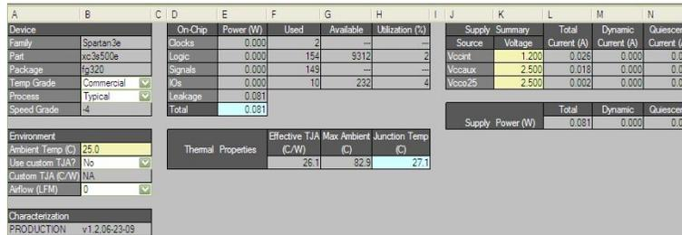
Figure 8. Power Supply Summary of Viterbi Decoder for K=3
