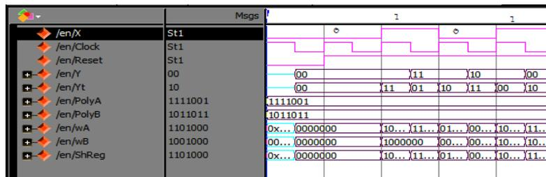
Figure 9. Simulation Result of Convolutional Encoder for K=7
