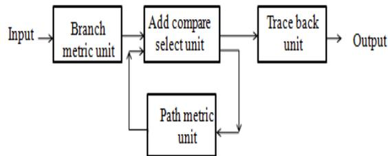
Figure 4. Block Diagram of Viterbi Decoder
