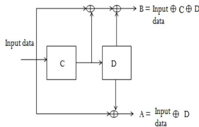
Figure 1. Convolutional Encoder for K=3
