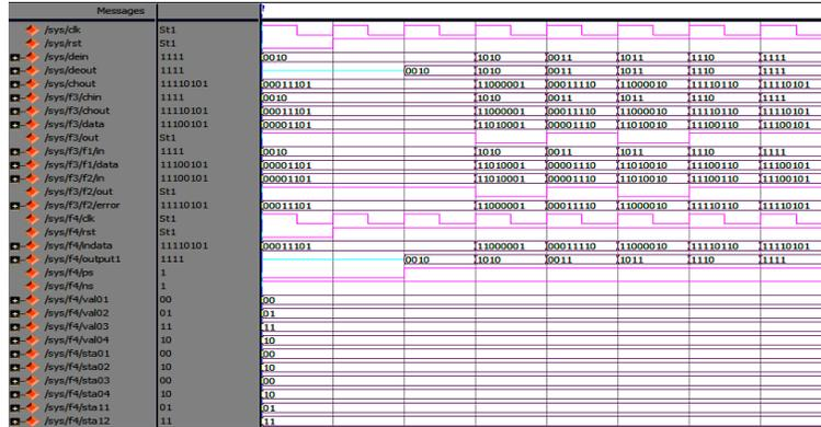
Figure 6. Simulation Result of Viterbi Decoder for K=3
