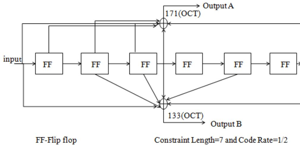
Figure 3. Convolutional Encoder for K=7
