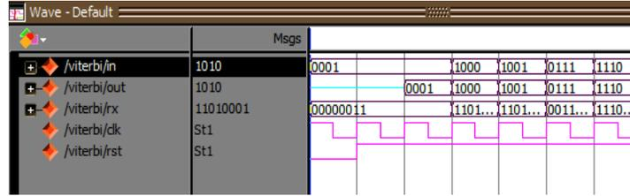
Figure 10. Simulation Result of Viterbi Decoder for K=7
