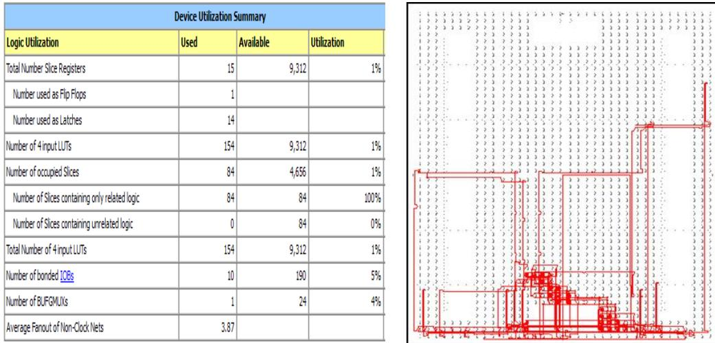
Figure 11. Device Utilization Summary and FPGA Editor of Viterbi Decoder for K=3
