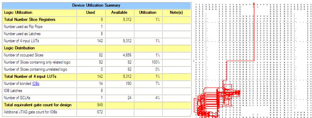
Figure 7. Device Utilization Summary and FPGA Editor of Viterbi Decoder for K=3
