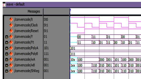
Figure 5. Simulation Result of Convolutional Encoder for K=3
