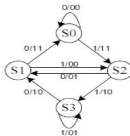
Figure 2. State Diagram of Convolutional Encoder for K=3
