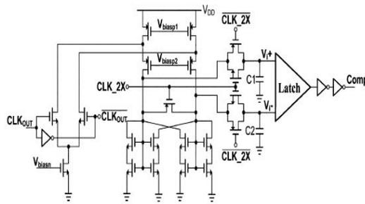
Figure 3. Duty Cycle Detector
