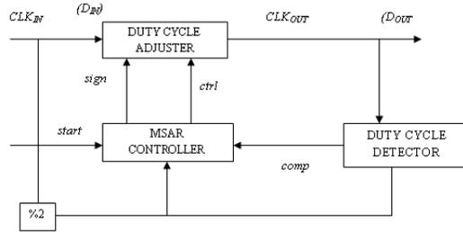
Figure 5. Block Diagram of the MSAR-DCC
