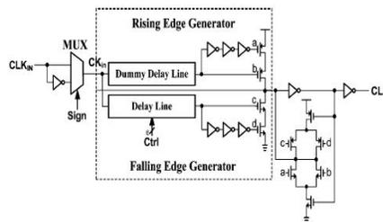
Figure 2. Duty Cycle Adjuster
