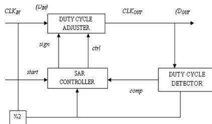
Figure 1. Block Diagram of the SAR-DCC
