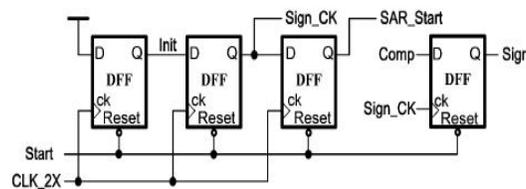
Figure 4. SAR controller with sign determination
