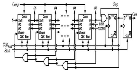
Figure. 6. 6-bit MSAR circuit
