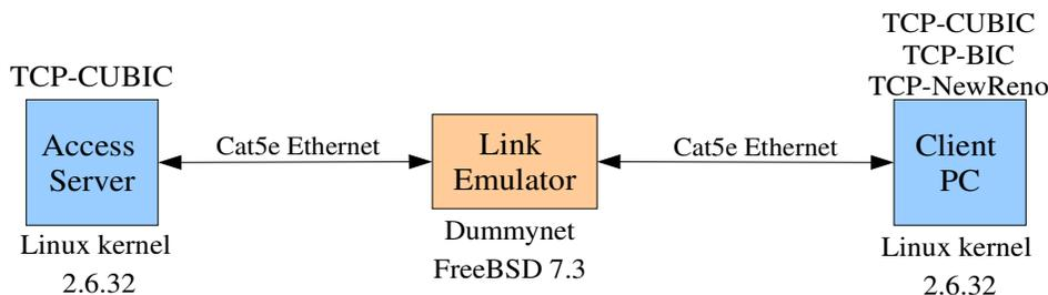
Figure 8: Network testbed for training and testing data collection
