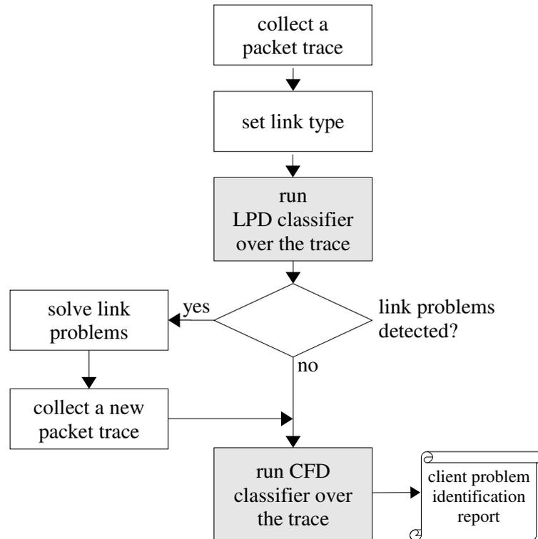
Figure 1: Overview of the operation of the IACD system
