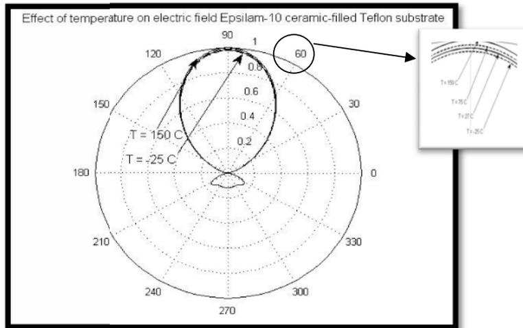
Figure. 29. Normalized electric field for different temperatures 150, 75, 27 and -25 °C. at  $\phi=0:2$  and  $\theta=0^0$  and radius of curvature 50 mm.
