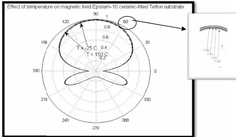
Figure. 30. Normalized magnetic field for different temperatures 150, 75, 27 and -25 °C. at  $\phi=0:2$  and  $\theta=0^0$  and radius of curvature 50 mm.
