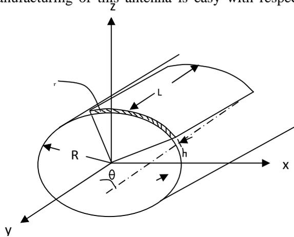
Figure 4: Geometry of cylindrical-rectangular patch antenna
