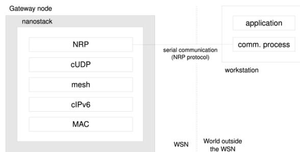
Figure 16: Node implementing Nanostack with NRP layer and serial communication to a workstation using NRP protocol
