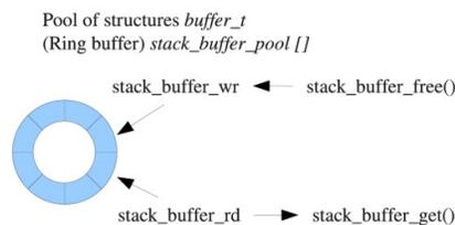
Figure 6: Ring buffer for *buffer\_t* instances.
