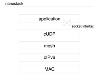
Figure 2: Principal Nanostack Layers
