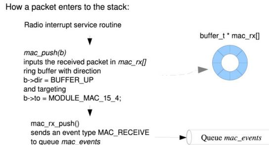
Figure 9: Details of packet entering to the stack
