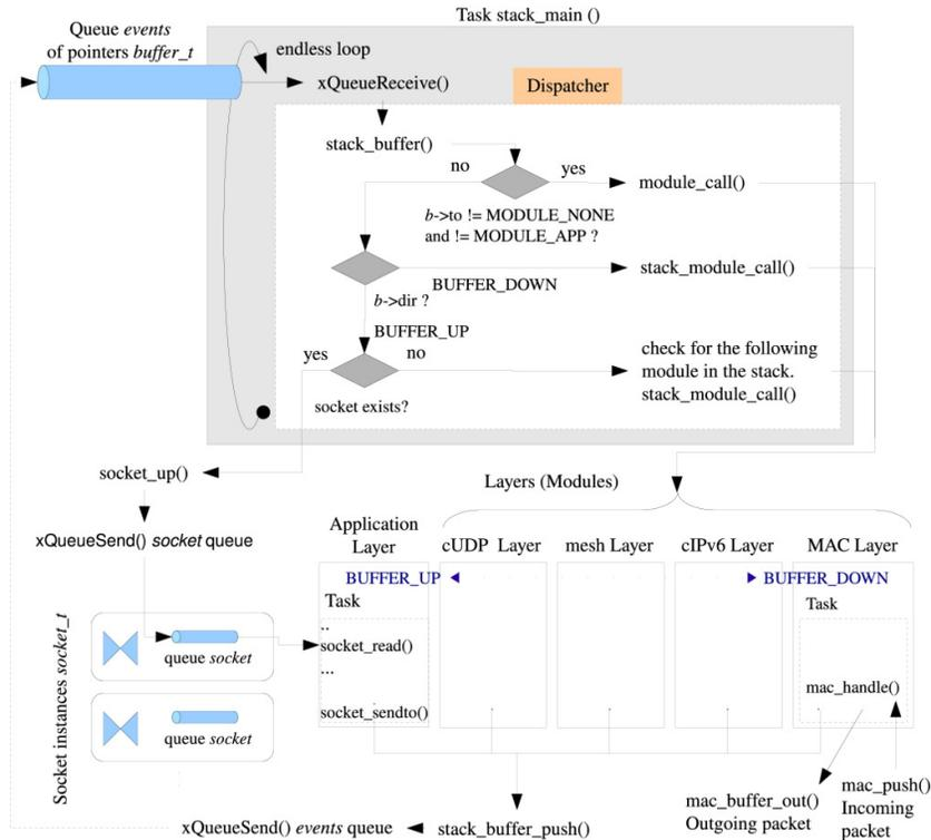
Figure 5: Nanostack architecture
