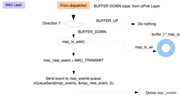
Figure 7: MAC layer module in the stack
