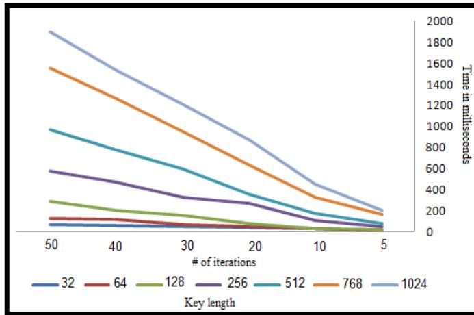
Figure 5. Column charts for key lengths and the computation time
