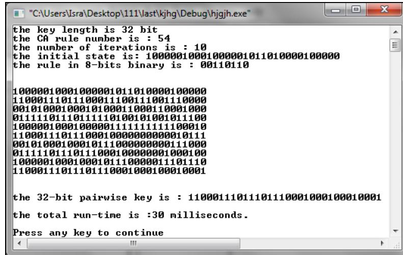
Figure 4. Establishing 32-bit key with 10 iterations based on CA rule 54
