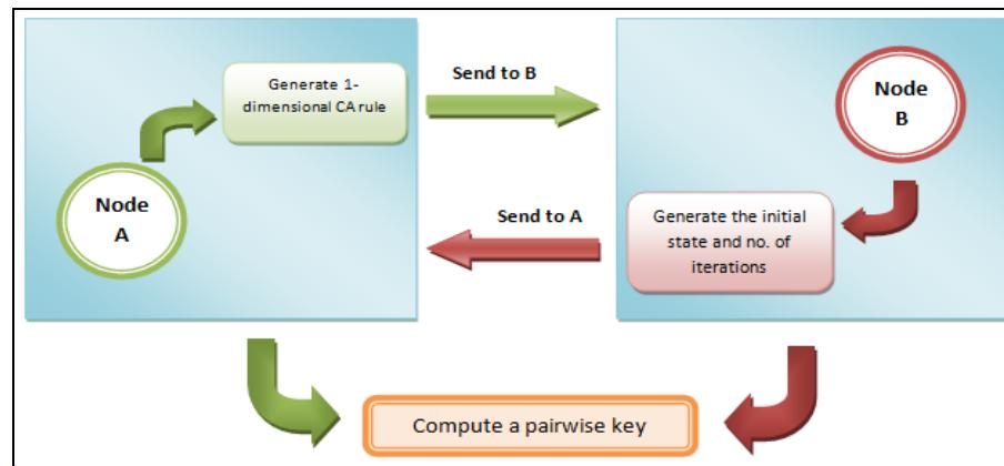
Figure 3. Pair-wise key-establishment between two nodes
