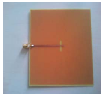
(a) (b) Figure 2. Fabricated Dielectric Resonator Antenna
