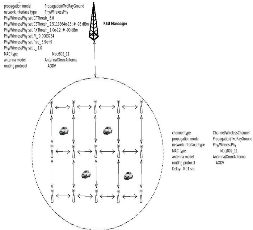
Figure 9. Network Simulation Setup
