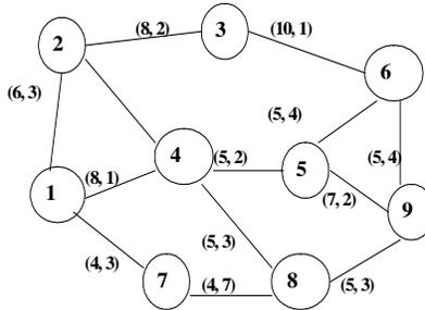
Figure 5: An Example Network With edges (Bandwidth, Delay)
