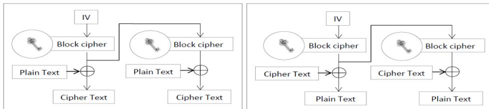
Figure 7: OFB mode encryption and decryption process.
