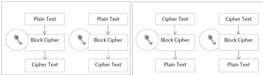
Figure 4: ECB mode encryption and decryption process.
