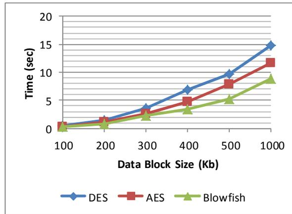
Figure 10: run time performance speed with CBC mode.
