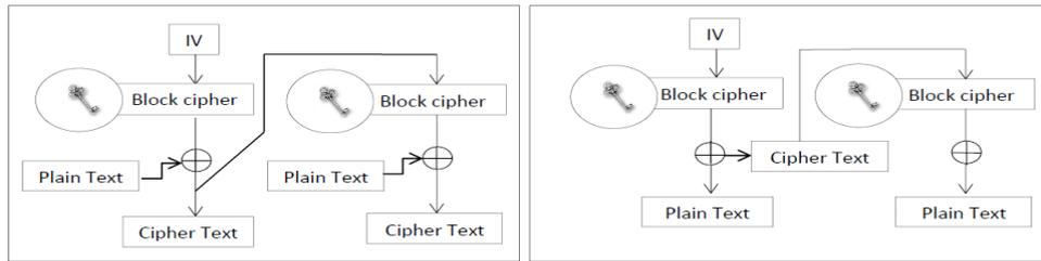
Figure 6: CFB mode encryption and decryption process.
