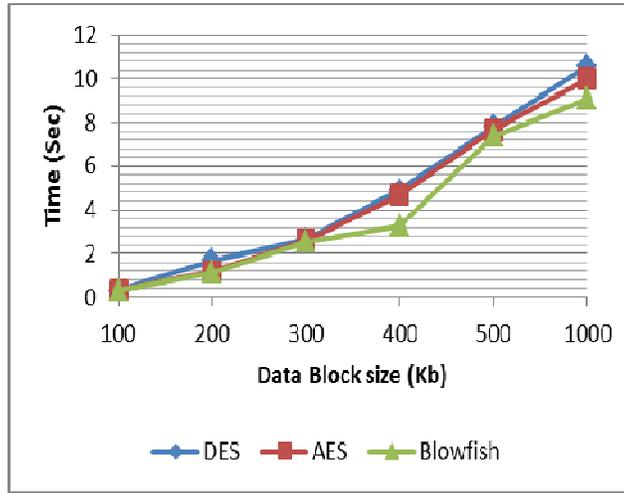
Figure 9: run time performance speed with ECB mode
