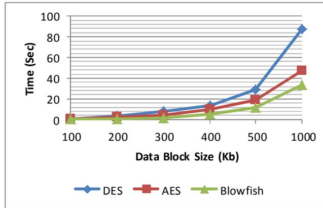
Figure 11: run time performance speed with CFB mode.
