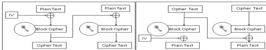
Figure 5: CBC mode encryption and decryption process.
