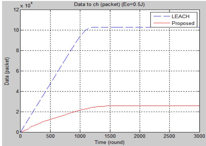
Figure 9. Data to CH between LEACH and proposed protocol (Eo = 0.5J)
