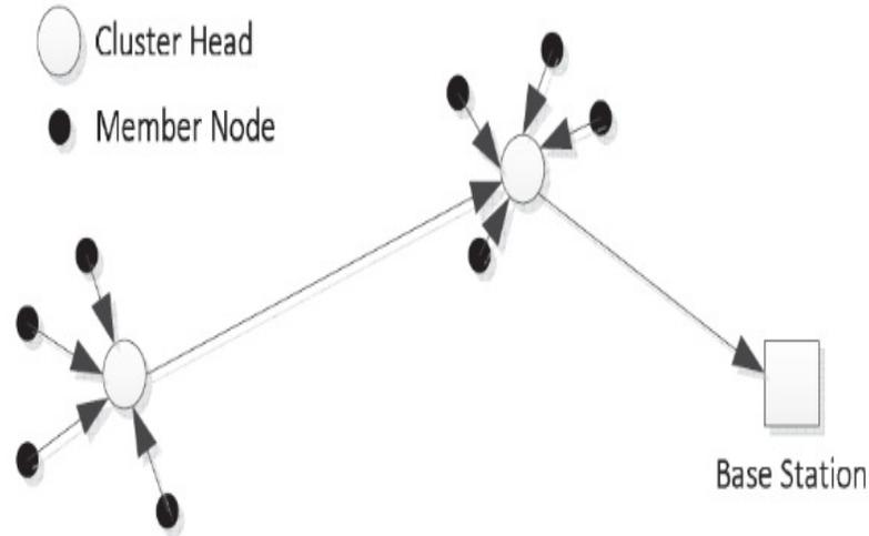
Figure 2. Transmit data in Multi-hop LEACH.
