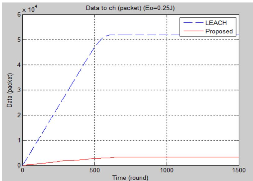
Figure 6. Data to CH between LEACH and proposed protocol ( $E_o = 0.25J$ )
