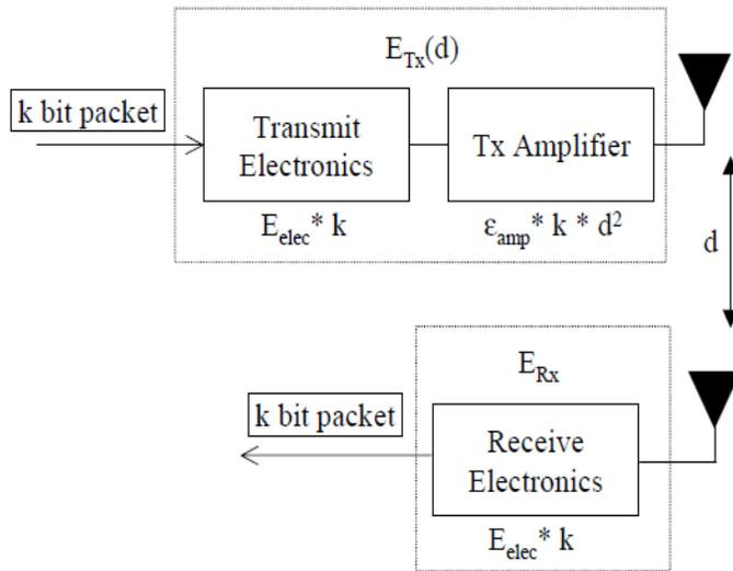
Figure 3. Energy model used in LEACH protocol
