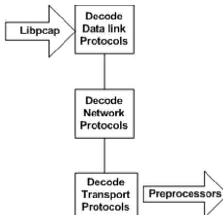
Figure 5. Packet decoder data-flow
