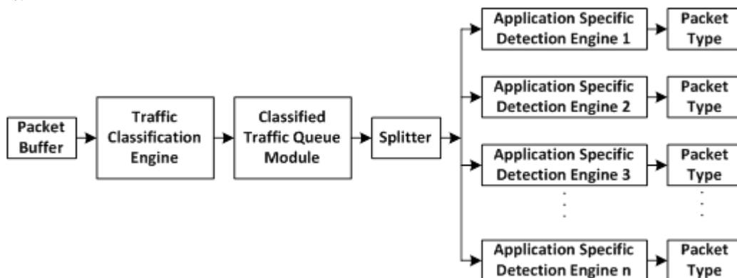
Figure 2. Pattern matching engine architecture
