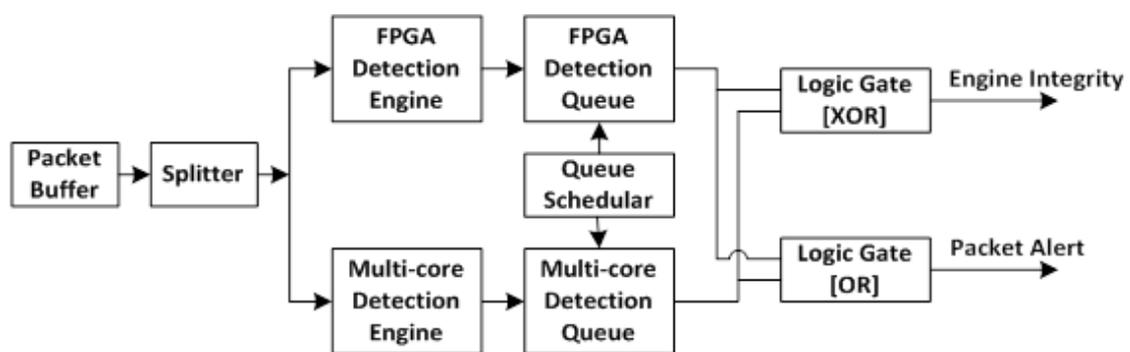
Figure 1. Trusted pattern matching engine
