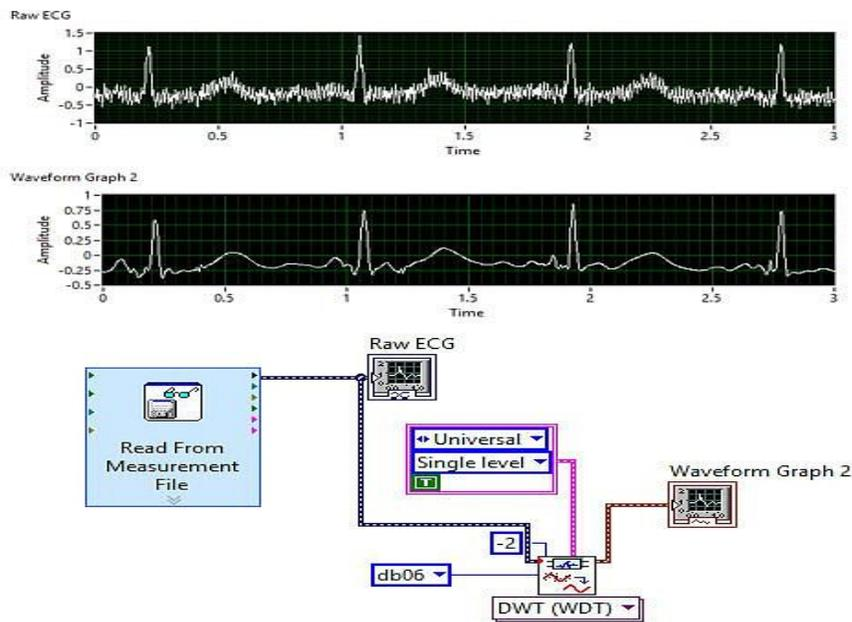
Figure 9. The ECG signal generated by our system with the Gaussian noise removed
