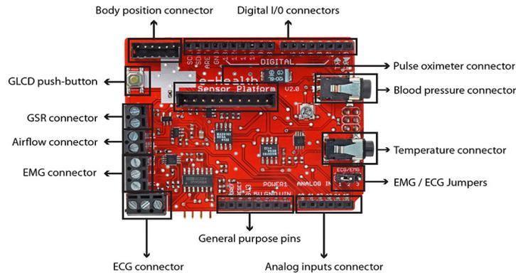
Figure 3. The biometric shield
