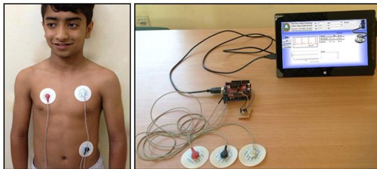
Figure 4. ECG Electrodes placements
