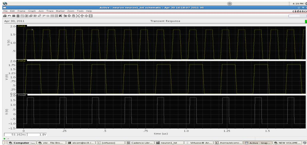
Fig 16(b): AND gate I/O waveforms
