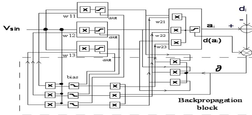
Fig.7 Neural network (1:3:1) with Backpropagation Algorithm
