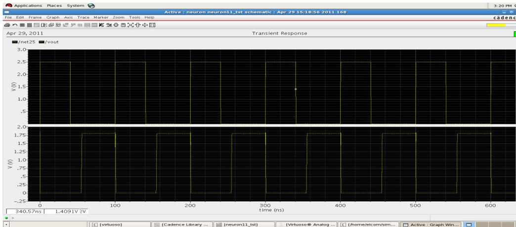
Fig 16(c): NOT gate I/O waveforms
