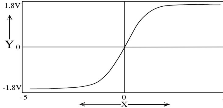
Fig.6 DC response of CMOS Differential Amplifier
