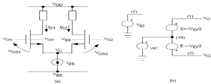
Fig.4 General MOS Differential Amplifier: (a) Schematic Diagram, (b) Input Gate voltage implementation.
