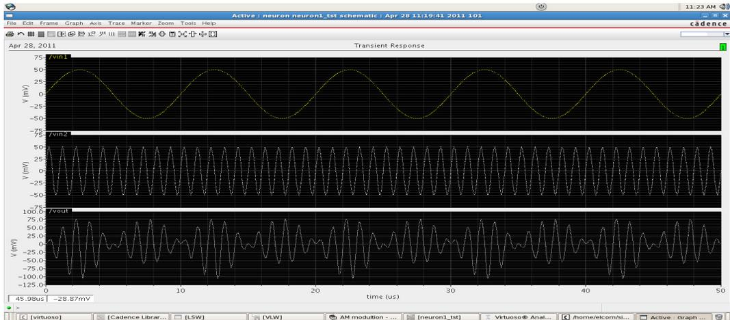
Fig 14: Transient Response of AM modulation
