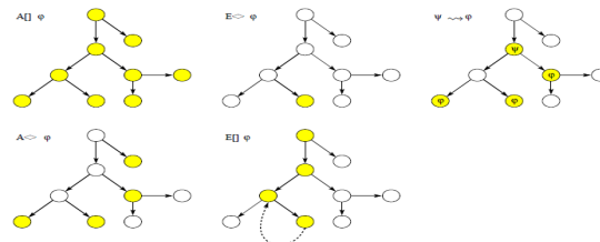
Figure 3: Path Formulae Supported in Uppaal. The Filled States Are Those for Which a Given State Formulae is True [14].
