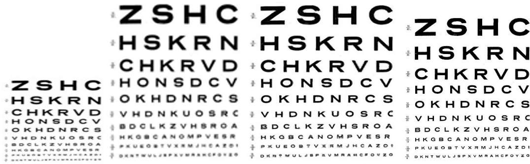
(a) Input (b) Bicubic interpolation (X3). (c) Unified single-image SR (x3) (d) Ground truth image. Figure 5: Comparison: The input image (a) was down-scaled (blurred and subsampled) by a factor of 3 from the ground-truth image (d). (b) shows bicubic interpolation of the input image (a) and (c) is the result of our unified single-image SR algorithm.
