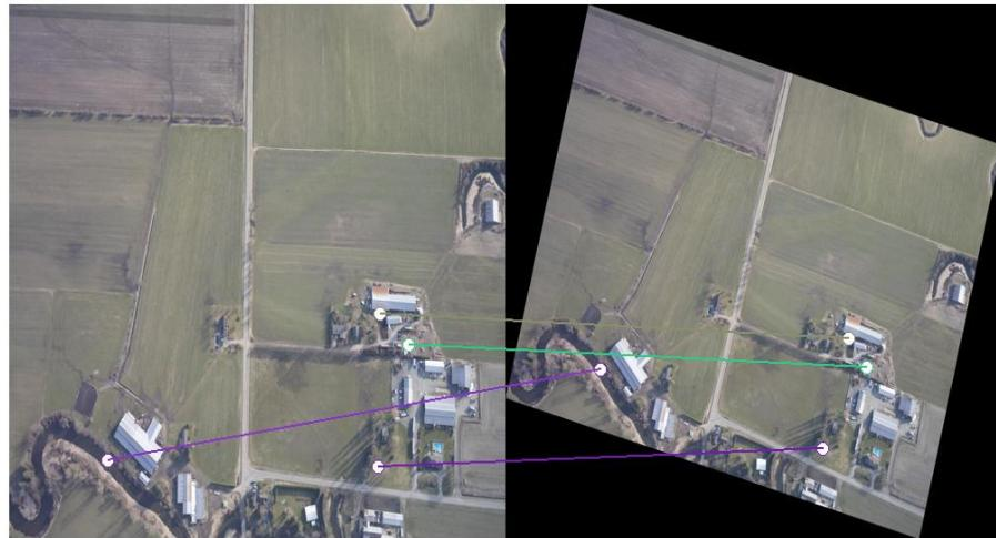
Figure 26. Descriptor length 64 with scale variation = 0.6 and rotation =15 and number of sample points 9x9
