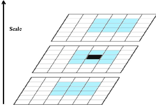
Figure 9. 3D non-maximum suppression concept for interest point localization
