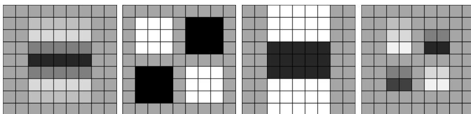
Figure 5. Discretized and cropped Gaussian and Box filter approximation for interest point detection
