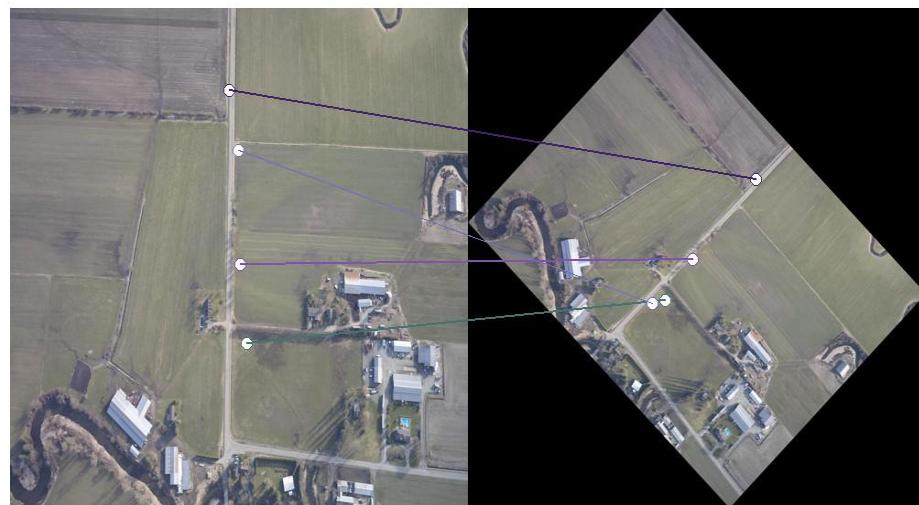
Figure 29 . Descriptor length 128 with scale variation = 0.8 and rotation =45 and number of sample points 5x5
