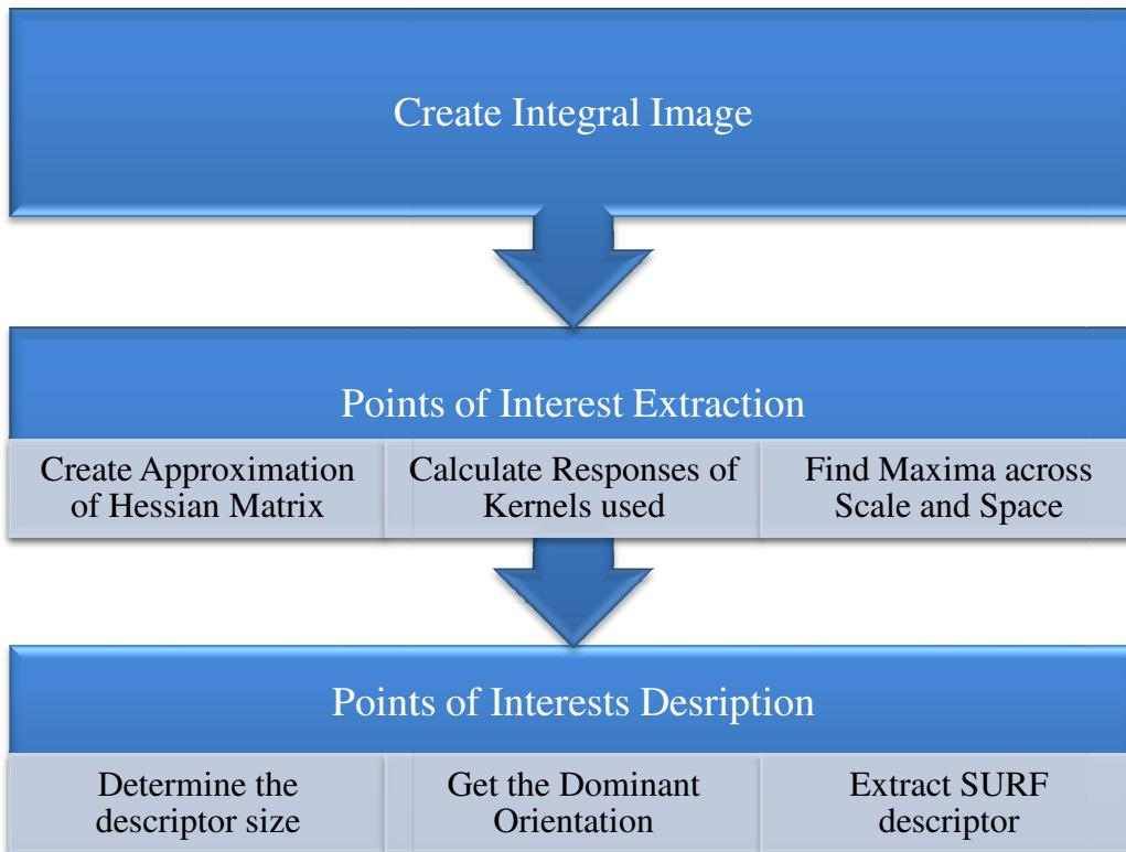
Figure 1.SURF block diagram
