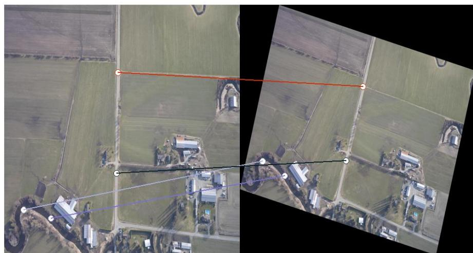
Figure 23. Descriptor length 36 with scale variation = 0.4 and rotation =15 and number of sample points 9x9
