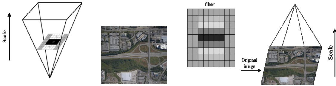
Figure 7. SURF implementation for scale space representation to the left where SIFT implementation is shown to the right
