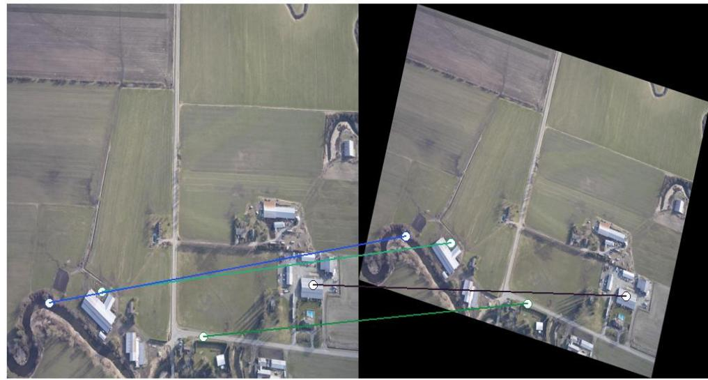
Figure 20. Descriptor length 36 with scale variation =0.2 and rotation = 15 and number of sample points 5x5
