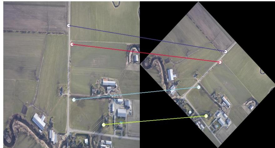
Figure 28. Descriptor length 64 with scale variation = 0.8 and rotation =45 and number of sample points 5x5
