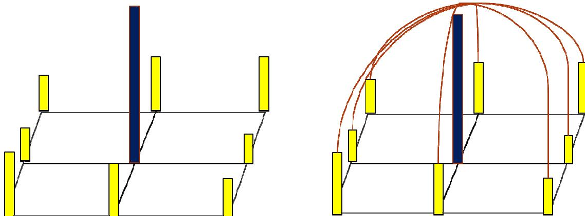
Figure 10.  $3 \times 3$  maximum blob response to the left and parabolic fitting maximum value to the right
