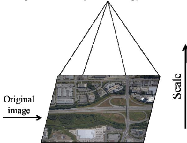
Figure 6. Image pyramid for scale space representation of an image
