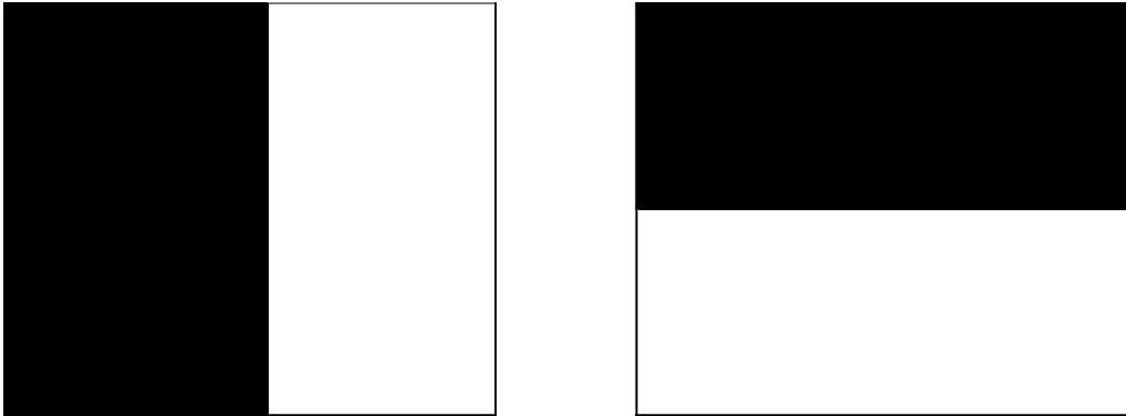
Figure 11. Haar wavelet filters used for computing the response in x direction (left) and y direction (right)
