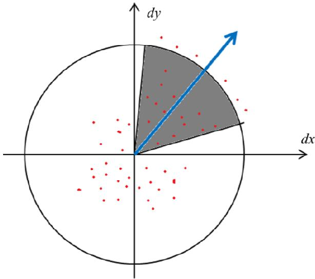
Figure 12. Sliding orientation window
