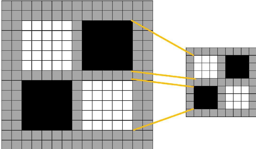
Figure 8. Filters  $D_{xy}$  for two successive scale levels ( $9 \times 9$  and  $15 \times 15$ )
