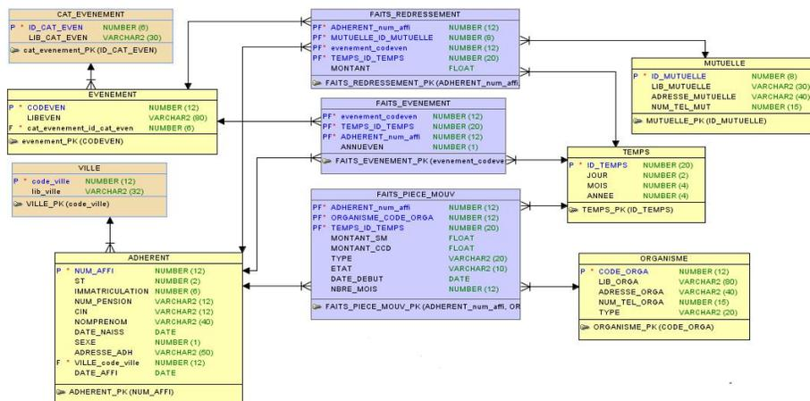
Figure 2 : Dimensional modeling –constellation schema
