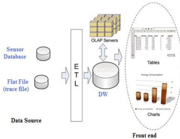
Figure 1 : Data Warehouse architecture
