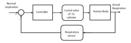
Figure 1: Closed Loop Control
