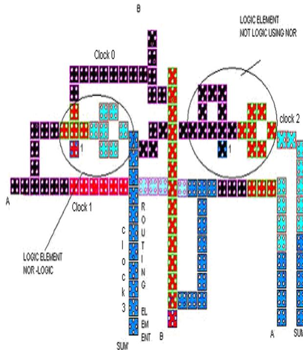
Fig. 4 QCA FPGA with sum function using NOR logic
