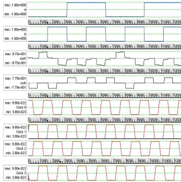
Fig.5 NOR logic implementation of QCA FPGA for sum function.
