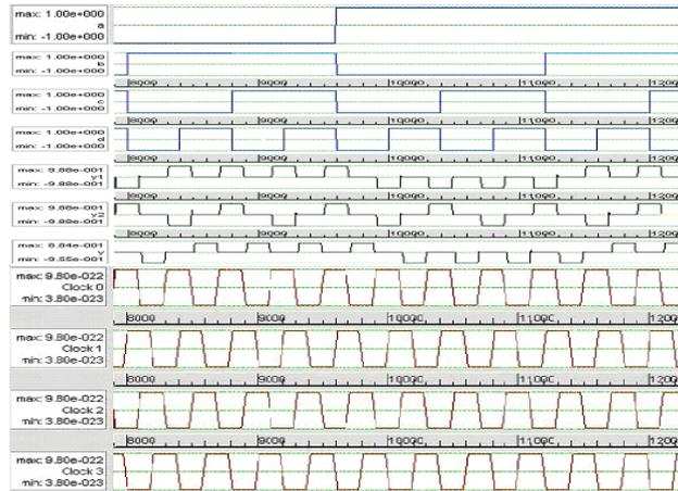
Fig.7 simulated waveform of QCA 4:1 MUX. Output Y is at Clock 0. with  $S_x = 1$  and  $S_0 = 1$ ,  $Y = b$ .
