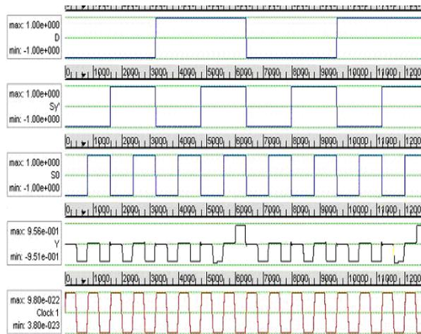
Fig.8 simulated waveform of equation 5 and 6 with setting D,  $S_y'$  and  $S_0$  as high to get 3 input AND gate.
