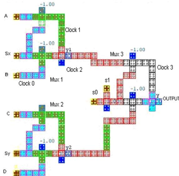
Fig.6 QCA cell 4:1 MUX
