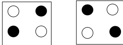
Fig.1 QCA cells with four quantum dots. 1.a  $P = +1$  (Binary 1) 1.b  $P = -1$  (Binary 0) [1][3][4][5]
