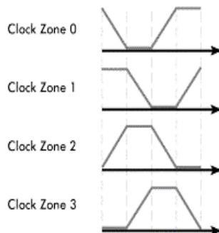
Fig.2 shows clocking scheme of QCA circuits [4][5][9][12.]
