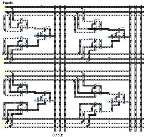
Fig.9 shows the 2 X 2 QCA FPGA using 4 : 1 MUX
