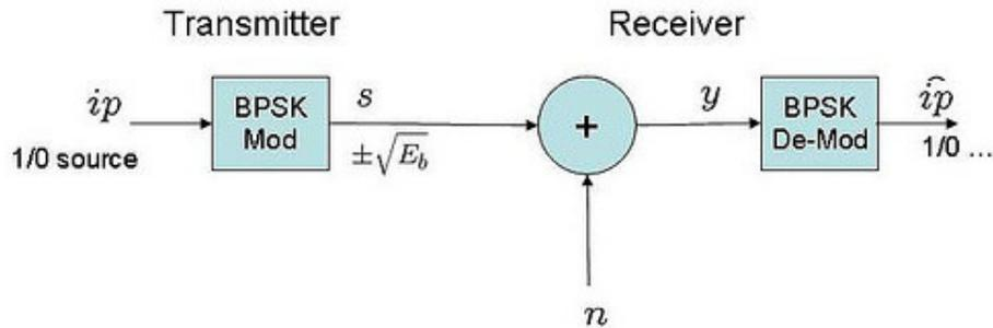
Fig.4 Simplified block diagram with BPSK transmitter-receiver
