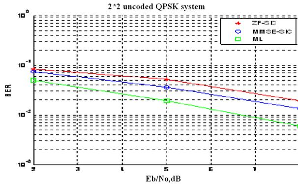
Fig.10 Comparison of ZF-SIC, MMSE-SIC and ML equalizer
