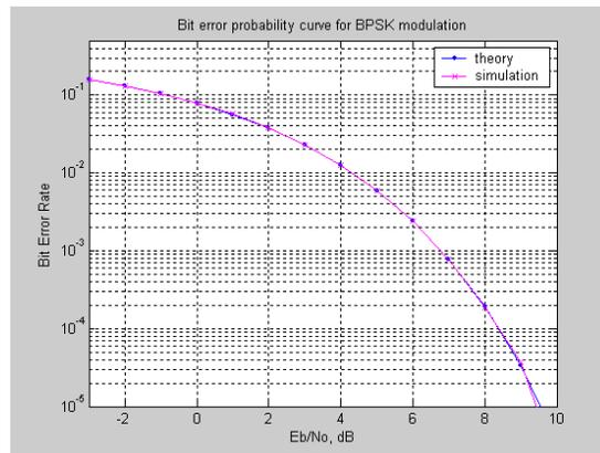
Fig.7 BER versus S/N for BPSK modulation
