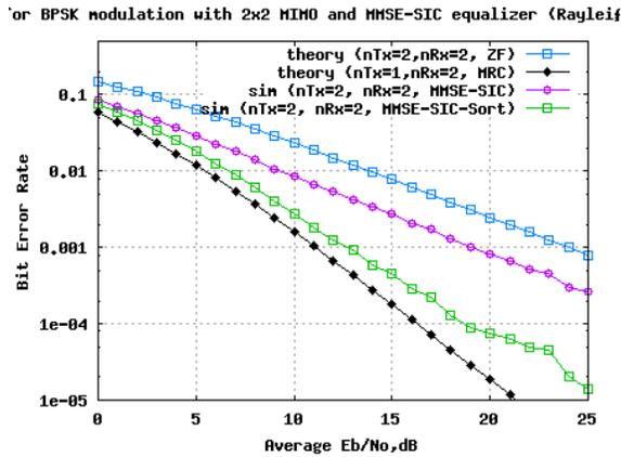
Fig.9 BPSK modulation with 2\*2 MIMO and MMSE-SIC equalizer
