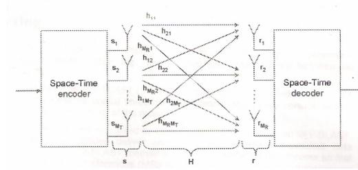
Fig.2. Physical MIMO channel
