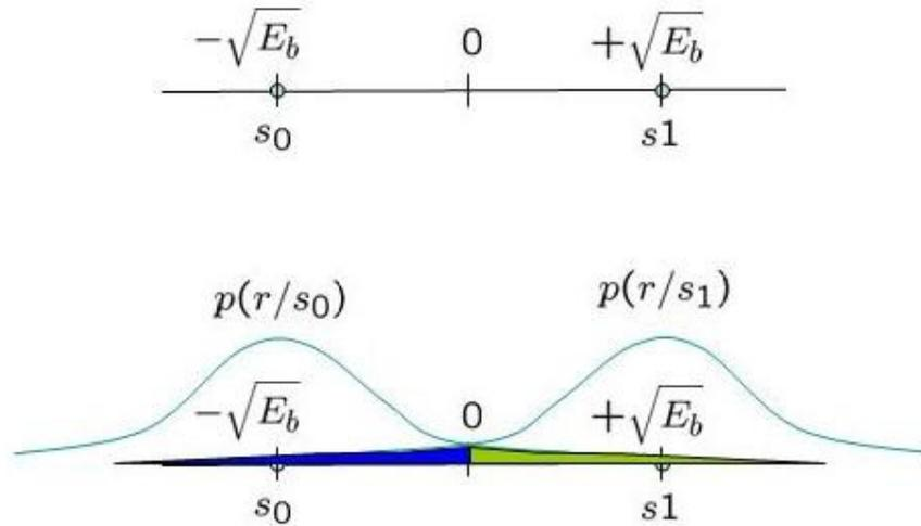
Fig.5 Conditional probability density function with BPSK modulation
