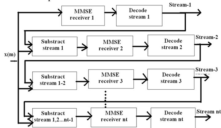
Fig.3 SIC using MMSE receiver
