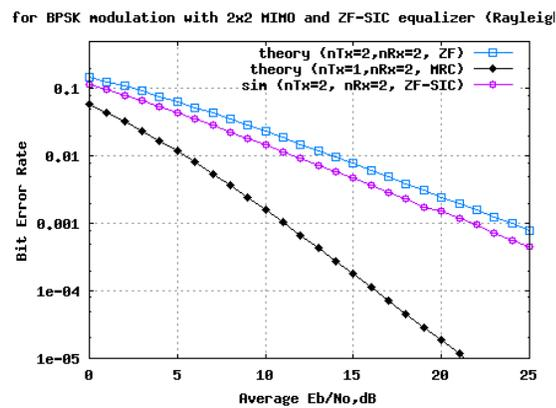
Fig.8 BPSK modulation with 2\*2 MIMO and ZF-SIC Equalizer
