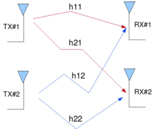
Fig.6 Transmit 2 Receive (2x2) MIMO channel
