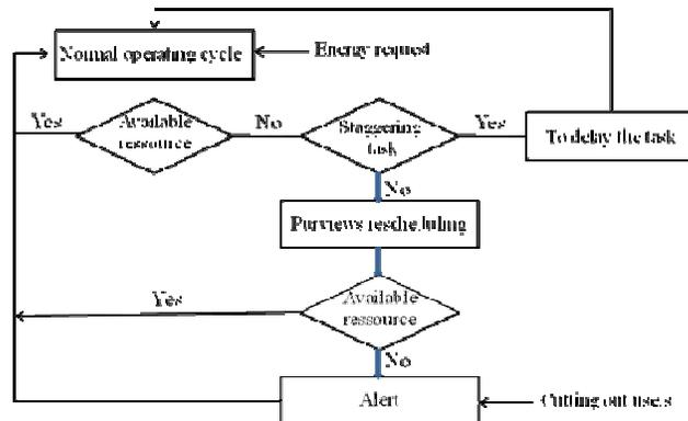
Figure 4. Real time scheduling algorithm
