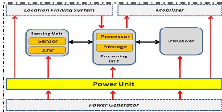
Figure 2. Basic physical architecture of an intelligent sensor
