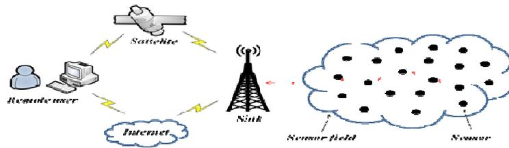
Figure 1. Basic architecture of a wireless sensor network.
