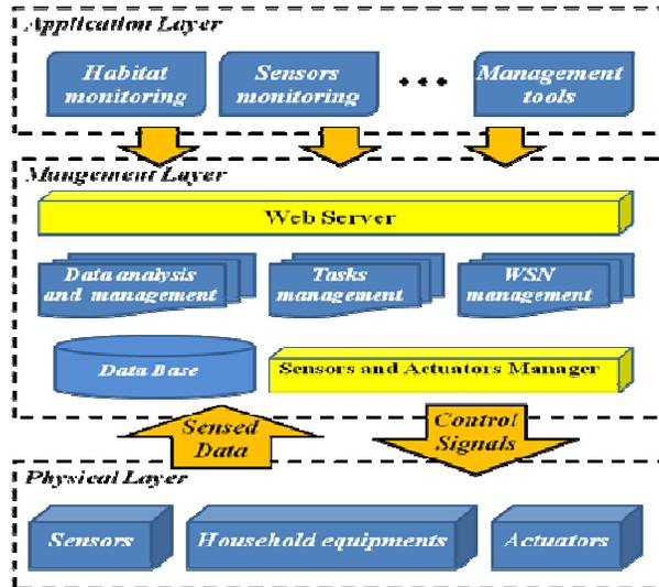
Figure 5. Physical structure of our platform
