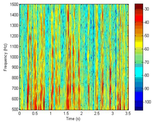
b.2 Spectrogram of encrypted signal before LPC
