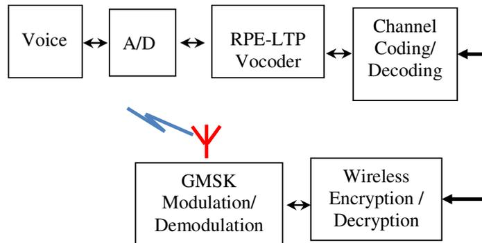
Figure 1. GSM voice transmission process.
