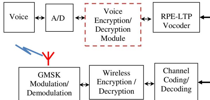
Figure 2. Voice encryption module access point in MT.
