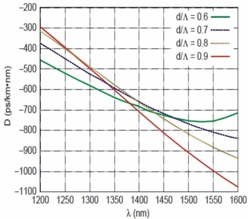
Fig. 5: Dispersion parameter for PCFs with  $\Lambda = 0.8 \mu\text{m}$  and different  $d/\Lambda$  values
