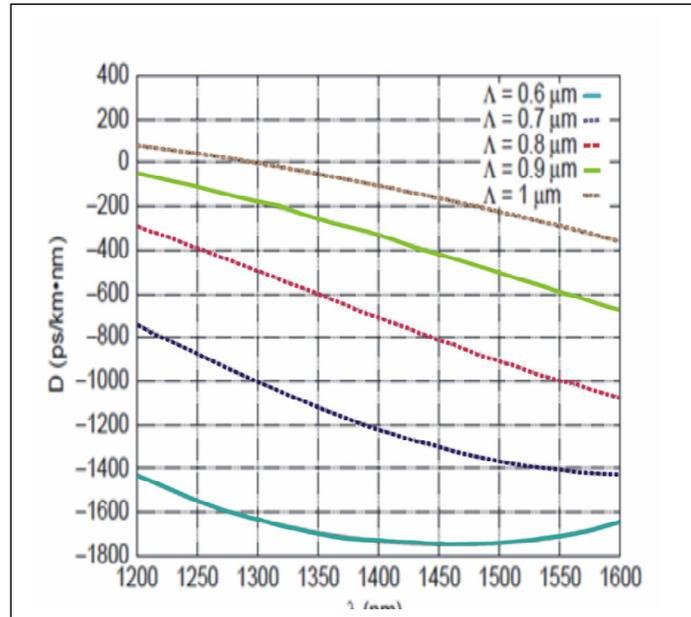
Fig. 4: Dispersion parameter for PCFs with  $d/\Lambda = 0.9 \mu\text{m}$  and different  $\Lambda$  values
