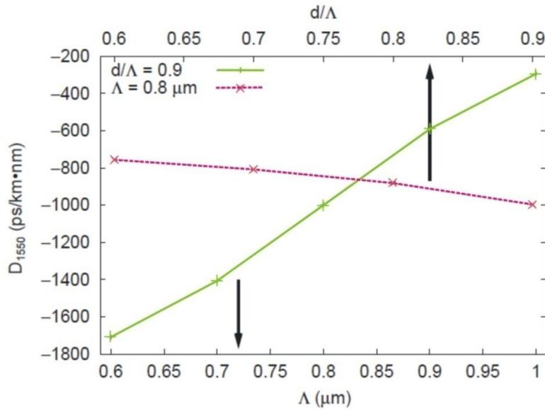
Fig. 6: Chromatic dispersion value at 1550 nm for the different triangular PCFs considered
