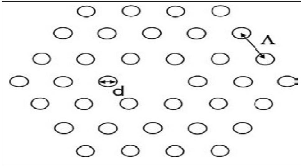
Fig. 1: Cross-section of a triangular PCF with the air-hole diameter  $d$  and the pitch  $\Lambda$ .
