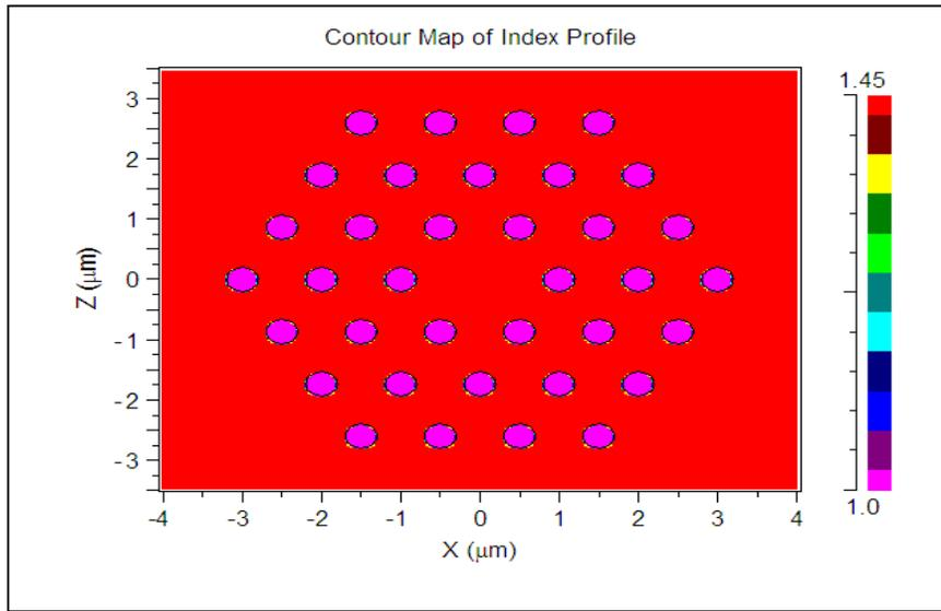
Fig.2 : Index profile of the triangular lattice PCF structure
