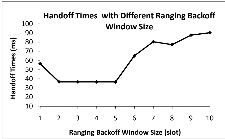
Figure 8. Handoff Times vs. Ranging Backoff Window Size
