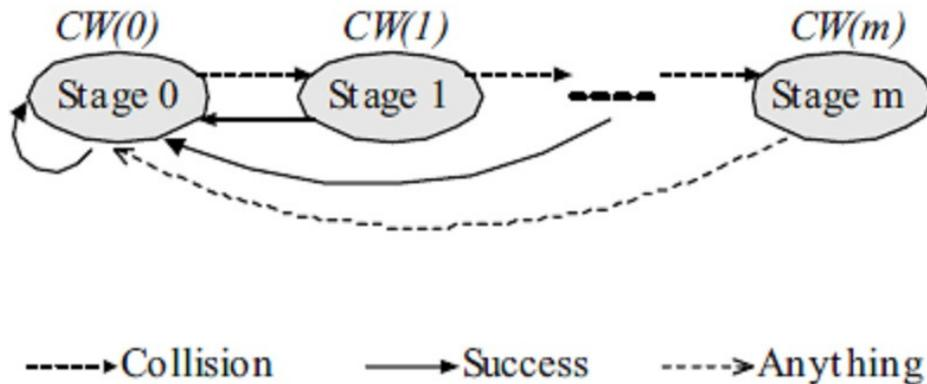
Figure 1.Operation of 802.11 DCF with BEB Algorithm
