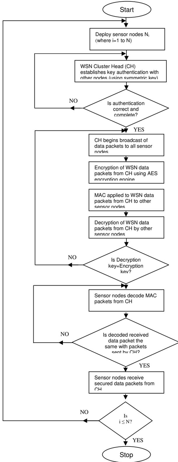
Figure 6. A process flowchart depicting the flow of securing WSN data packets from WSN cluster head (CH) to other nodes using authentication keys, encryption and MAC
