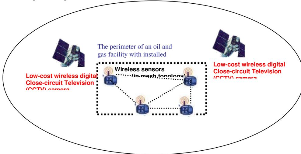
Figure 4. Deployment architecture for wireless digital Close-Circuit Television Circuit (CCTV) to provide surveillance for an oil facility in Niger Delta region
