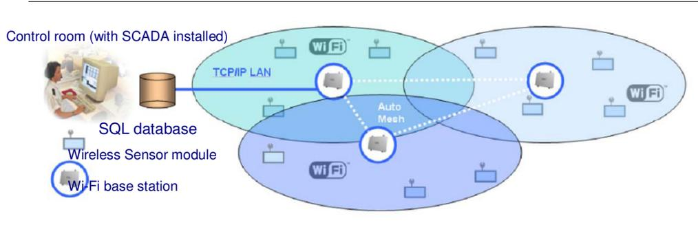
Figure 3. *Direct connection between wireless sensor network and SQL database using Wi-Fi network base station to facilitate easy and fast reporting of vandalism to the control room (Source from [14])*
