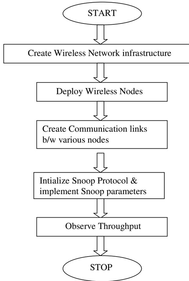
Fig. 2 Simulation setup flow diagram
