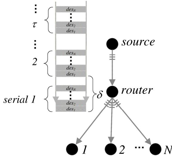
Figure 2: The mechanism for passive tomography with source and N end hosts.
