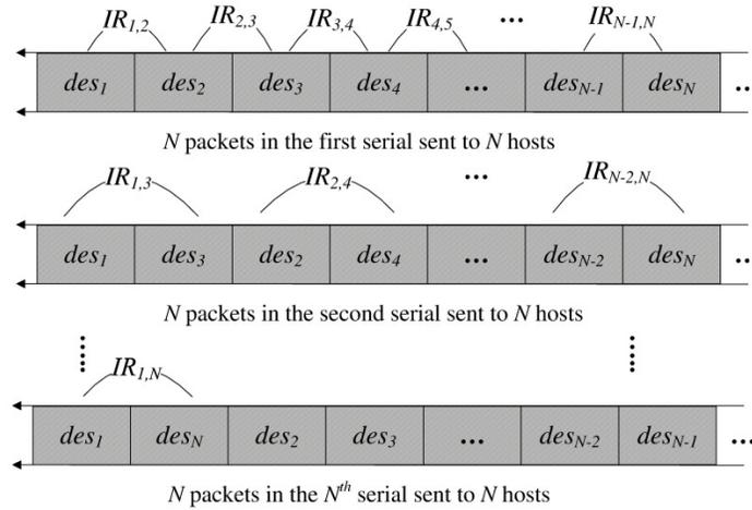
Figure 3: Arrangement of  $IR$ .  $IR_{i,j}$  in each serial indicates blocks destined to  $i, j$  should be successive.
