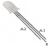
Figure 1. Bicolor LED (Model: SSL-LX5097IGW)
