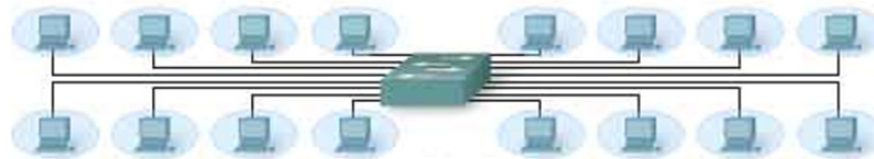
Figure4: LAN network using Ethernet Switch.
