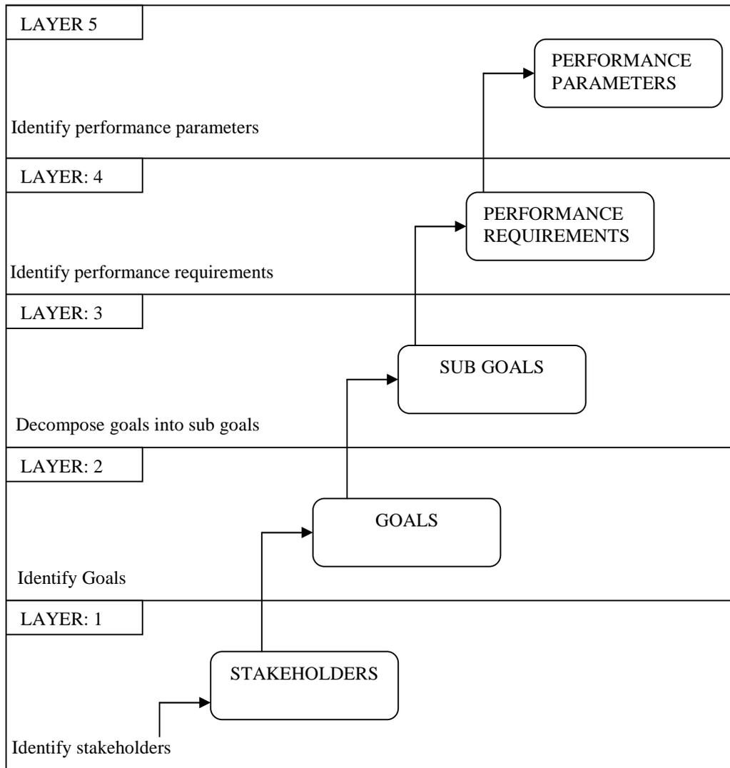
Fig 1: General Architecture for Five layered model for Performance requirements identification
