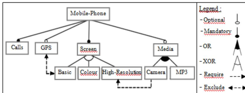
Figure 1. Feature diagram of a mobile phone product line
