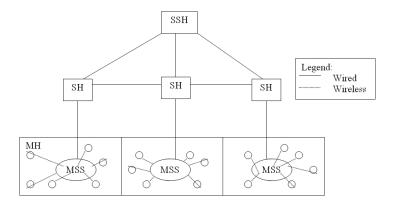
Figure 1: Four-layered Mobile Cellular Network Architecture
