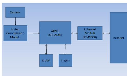
Figure 2 Block Diagram of ENVMT using ARM
