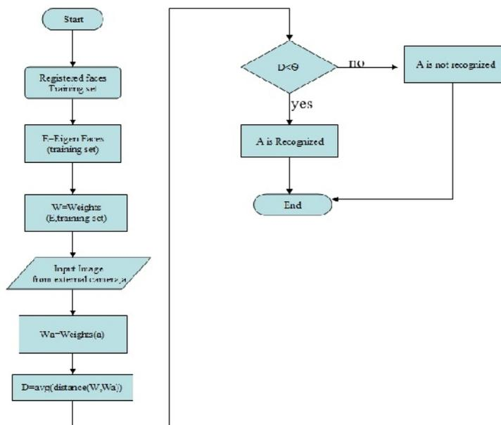
Fig 8. Face recognition using eigen face approach
