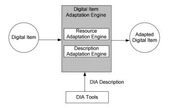
Figure 9: Concept of MPEG-21 DIA
