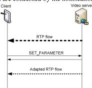
Figure 11: Message flow of renegotiation process
