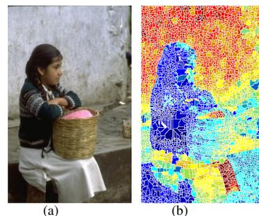
Figure 2. Watershed Transform; (a) Original image, (b) watershed applied
