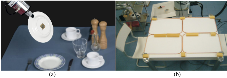
Figure 6. RFID tags implanted on the dishes (a) and the Tag Reader installed on the table (b)
