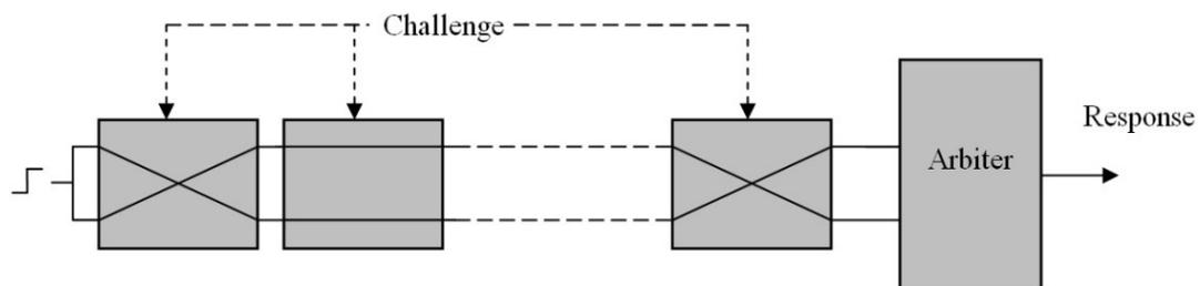
Figure 4. Arbiter PUF architecture
