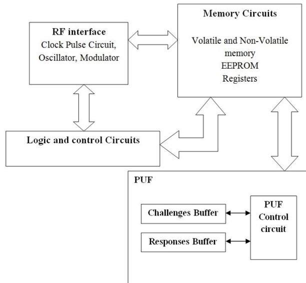
Figure 7. PUF-enabled RFID tag
