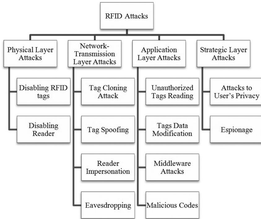
Figure 2. RFID Layer Attacks
