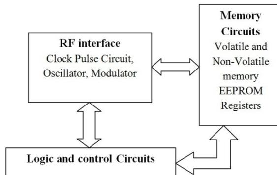
Figure 6. Components of RFID Architecture
