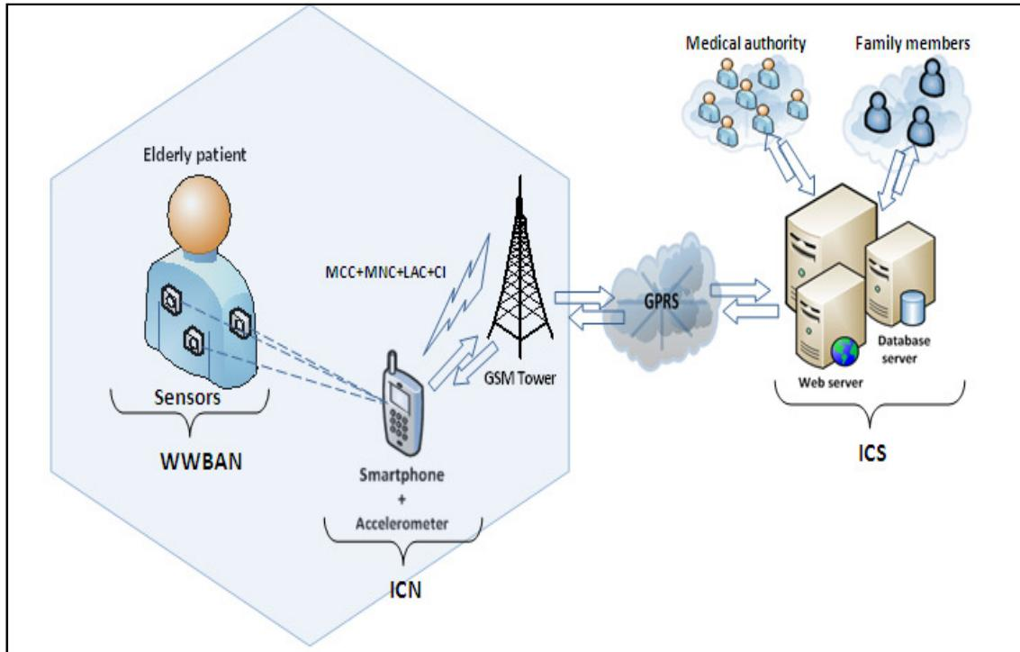
Figure1. UMHMSE System Architecture
