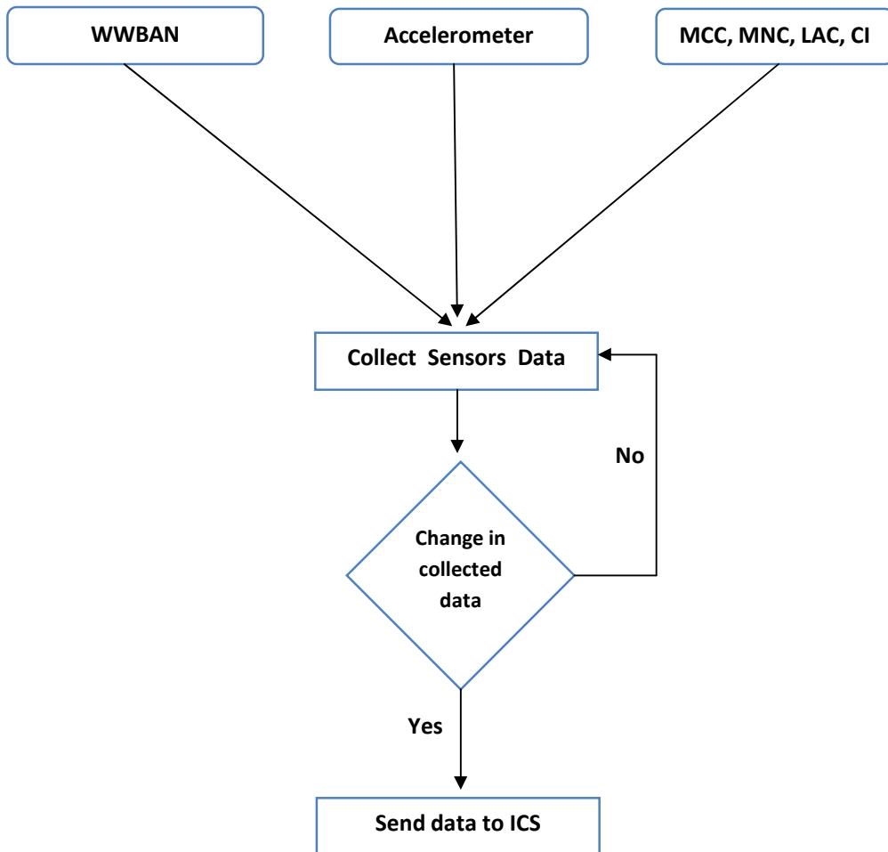
Figure 3. Flow diagram of the ICN function
