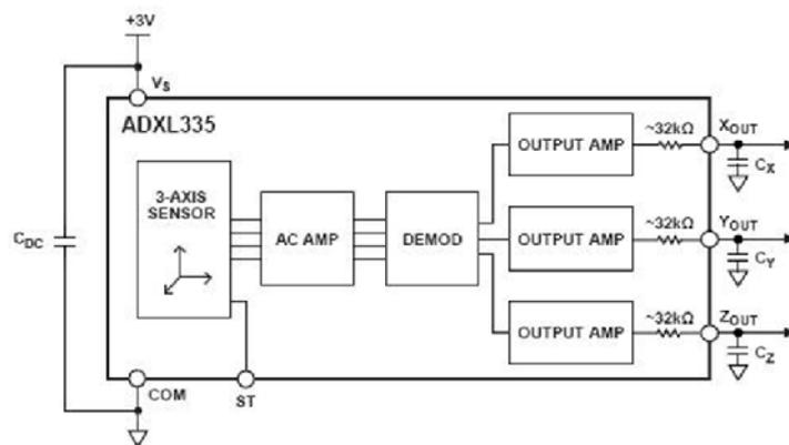
Figure 3. The schematic diagram of ADXL335
