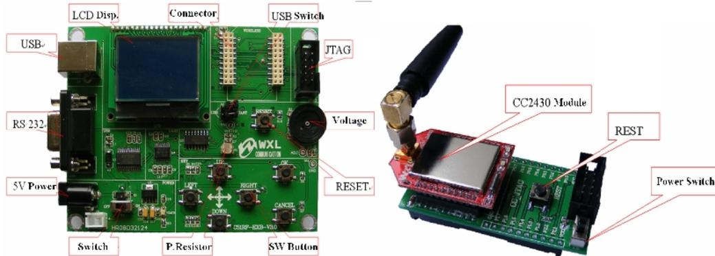
Figure 5. EB and CC2430EM+BB module
