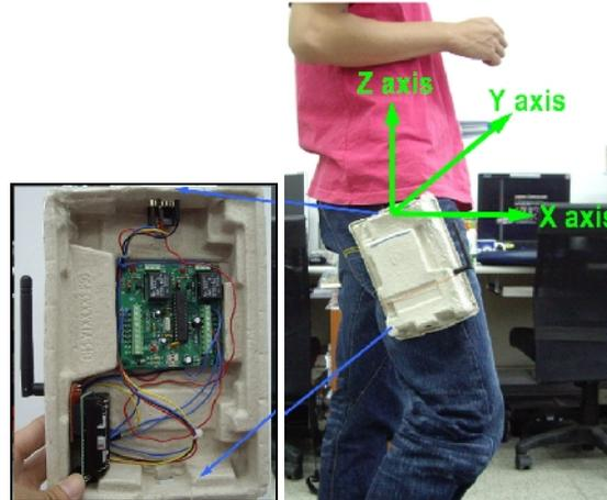
Figure 11. The user wearing the posture recognition module
