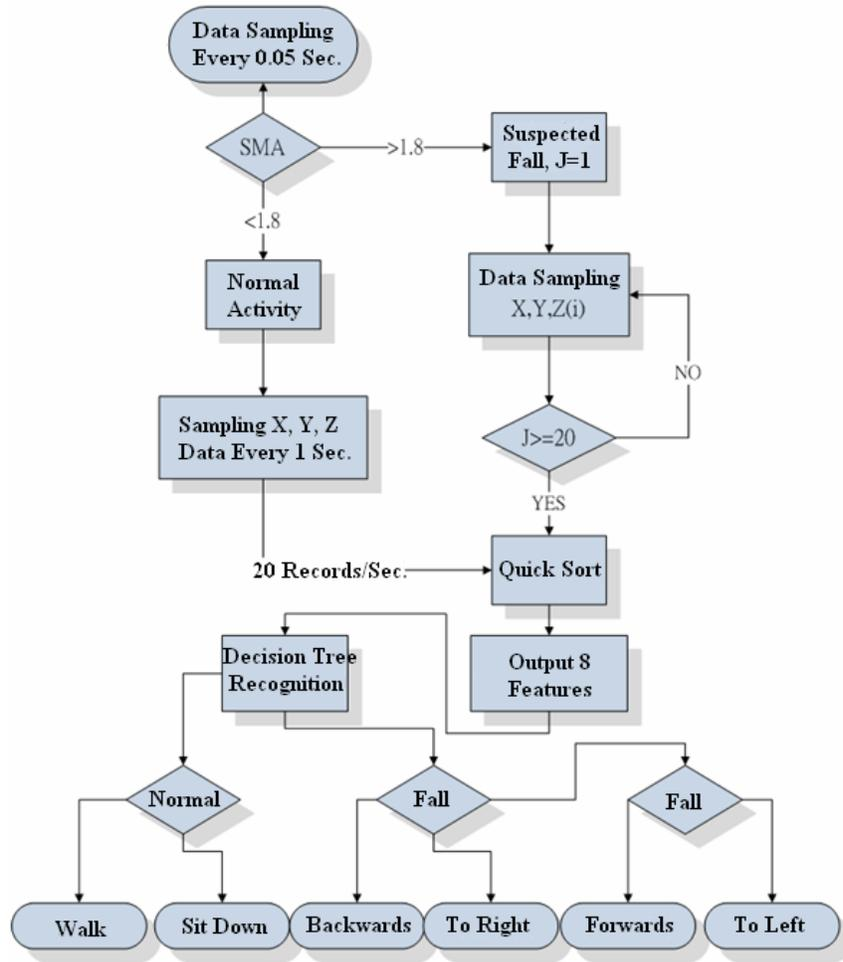
Figure 10. Feature extraction and identification procedure
