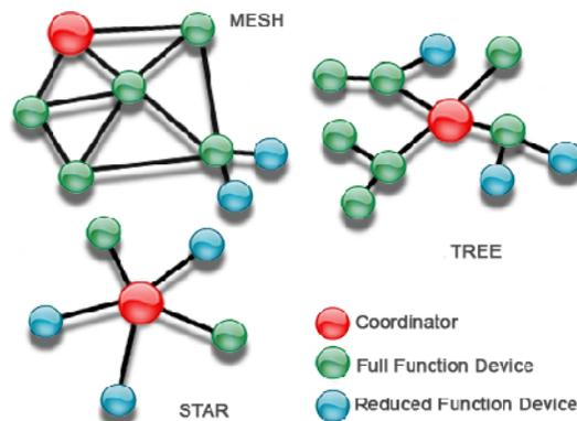
Figure 1. ZigBee's three network architectures
