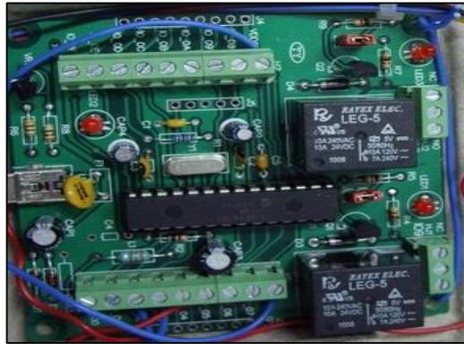
Figure 4. PIC18F24J microcontroller module used in this study
