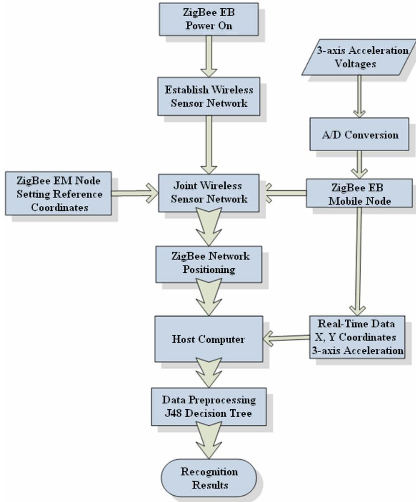
Figure 9. Operating procedure of activity monitoring system
