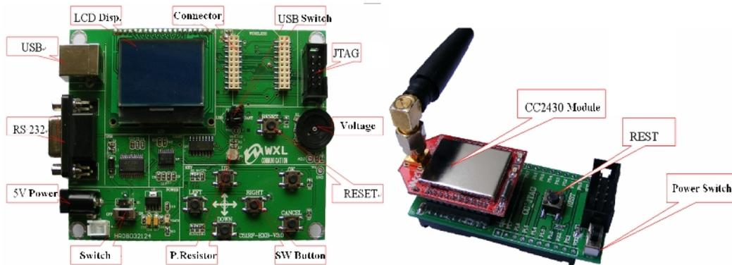
Figure 5. EB and CC2430EM+BB module
