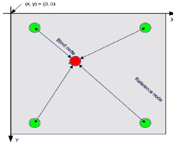
Figure 6. The RSSI ZigBee positioning method
