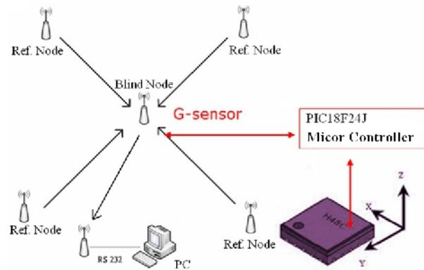
Figure 2. The activity monitoring system using G-sensors
