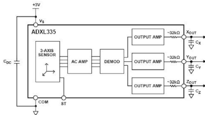
Figure 3. The schematic diagram of ADXL335
