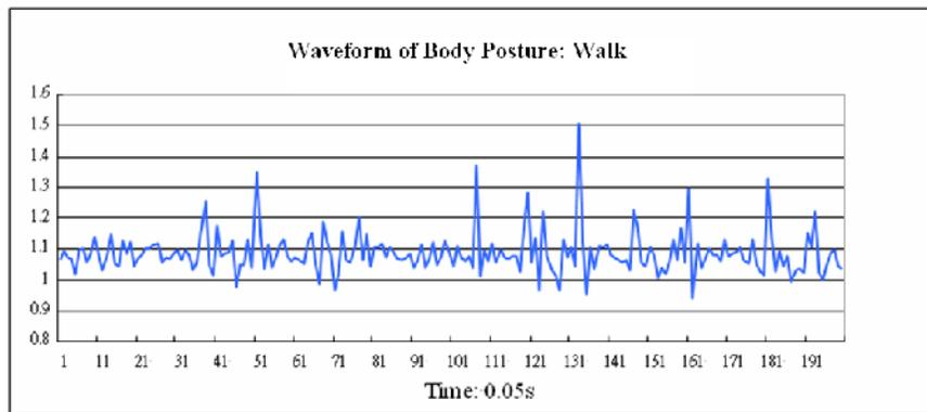
Figure 13. The SMV waveform for the walk posture
