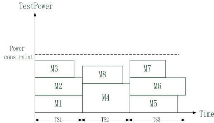
Fig. 1 . An example of test grouping results of 8 memories
