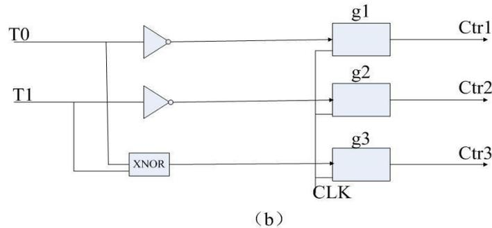
Fig.4. (a) A gated distributed BIST structure with encoder (b) Encoder and gating circuit
