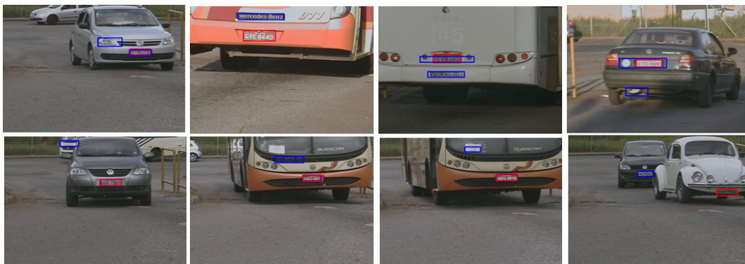
Fig. 10. Example of detections for hybrid [9] (top row) and sliding window using HOG features (bottom row) approaches.
